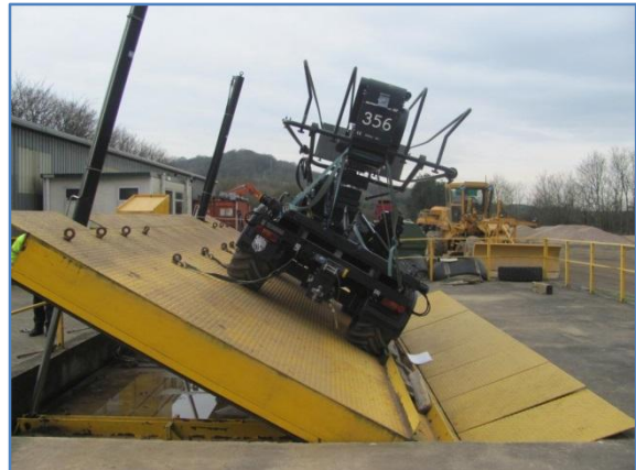
Figure 6 - Config. 2, Rear View, 29.2° Platform
