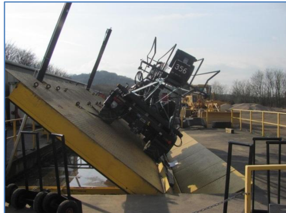
Figure 14 - Config. 6, Rear View, 38.2° Platform
