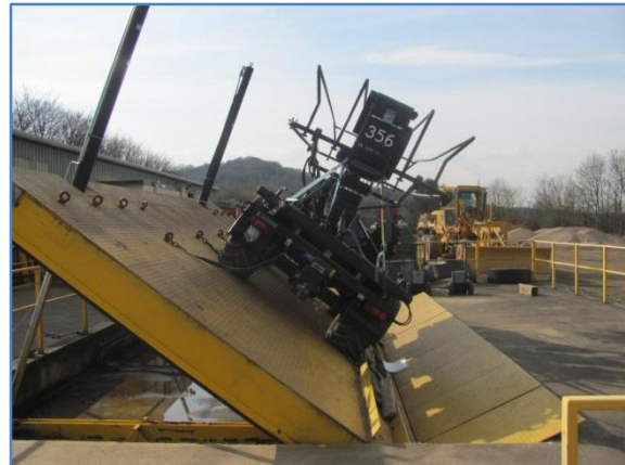
Figure 10 - Config. 4, Rear View, 36.1° Platform
