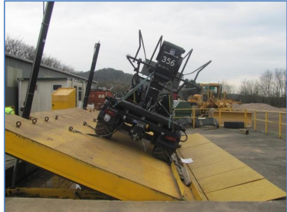
Figure 4 - Config. 1, Rear View, 20.5° Platform
