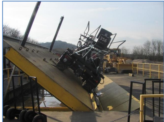
Figure 14 - Config. 6, Rear View, 38.2° Platform
